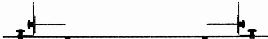
Abb. 1: Reflect Port 1 und Reflect Port 2 Kalibrierstandards Fig. 1: Reflect Port 1 and Reflect Port 2 calibration standards
