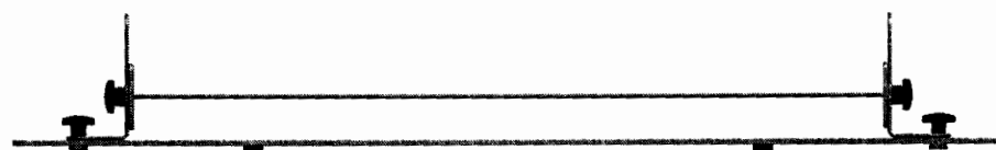
Abb. 4: Line 2 Kalibrierstandard Fig. 4: Line 2 calibration standard
