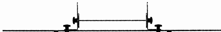
Abb. 3: Line 1 Kalibrierstandard (für hohe Frequenzen) Fig. 3: Line 1 calibration standard (for high frequencies)
